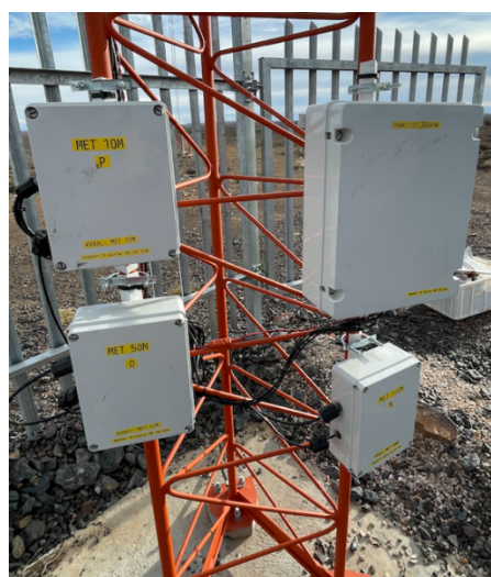
Figure 2: Bat monitoring equipment on the met mast
